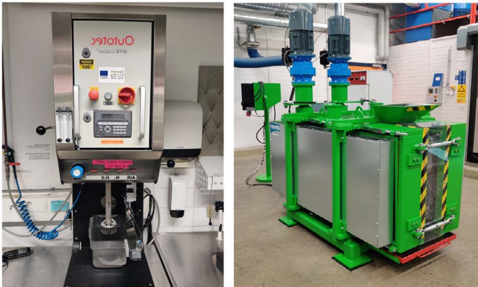
Fig. 2. Novel processing technologies developed by Oulu Mining School: continuously compressing and crushing (CCC) system (left) and advanced flotation cell (right) for efficient REE ore processing.
